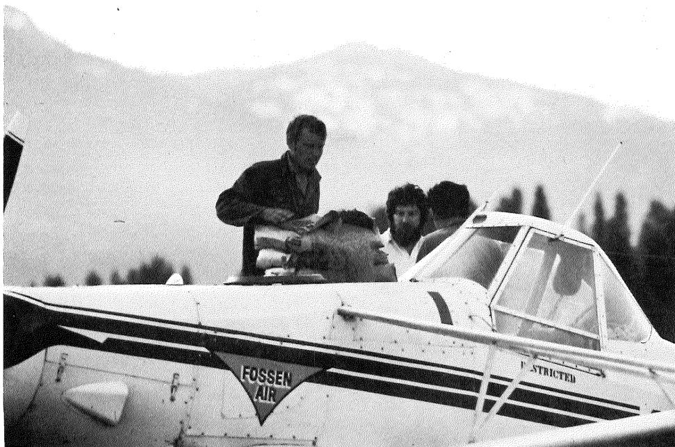
16. Aerial application of both seed and fertilizer was undertaken by Fossen Air using a Piper P. A. 25 Pawnee.
